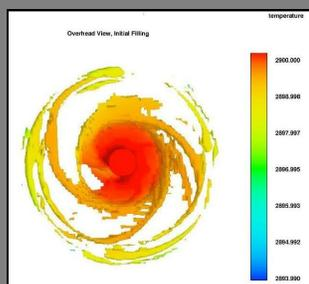
technology has advanced to the point that many models now take hours or less to get initial results, making it economically feasible to simulate even lower quantity casting applications. One major advance in the technology unique to MetalTek is the ability to accurately simulate the fluid dynamics and thermal dynamics of the molten metal within the rotating centrifugal mold cavity. This allows the engineer to predict, and mitigate
