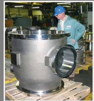
The finished cost of a component cast as a shaped centrifugal may be considerably lower than for a straight walled component because greatly reduced machining costs can more than offset the slightly higher mold and processing costs of a shaped centrifugal. For example, one MetalTek customer converted a straight walled forging to a net shaped centrifugal and eliminated eight weeks of machining on a five axis mill, significantly reducing the component cost, while maintaining product quality.
